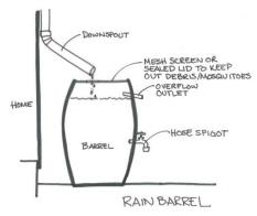
Rain barrel diagram
